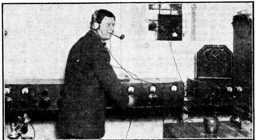
EMPIRE BROADCAST RECEPTION. Although Mr. Gerald Marcuse, seen in the photograph, is mainly concerned with transmission from his well-known station 2NM, he finds time to maintain an efficient receiving equipment. The receiver above is a short-wave superheterodyne which brings in Australian stations on the loud-speaker.
