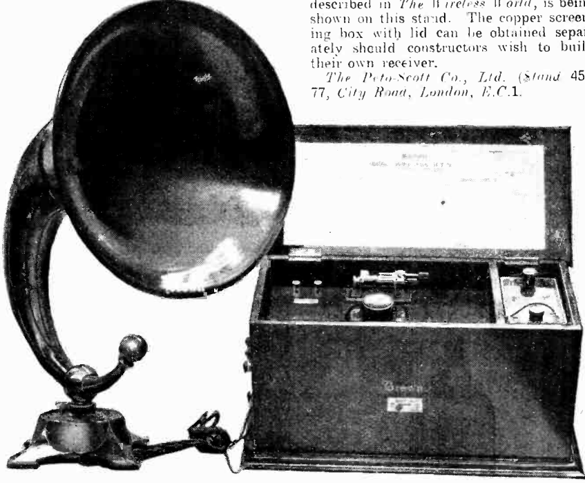
Valve crystal receiver with valveless amplifier.
